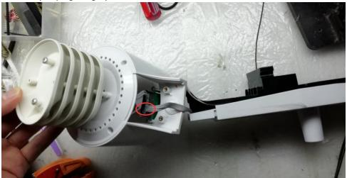
3. Repeat the operation for the original sensor array and plug the grey cable into the replacement sensor array as indicated;
